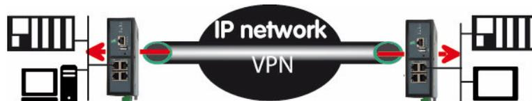
The router which initiates the connection is called the VPN client
